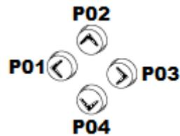
Figure 90: The cursor buttons are wired in the circuit diagram as contacts P 01 to P 04.
